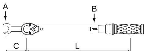
A number of variables including the length of the adapter or extension, length of the wrench and variations in hand position on the wrench will affect the accuracy of the above calculation.
